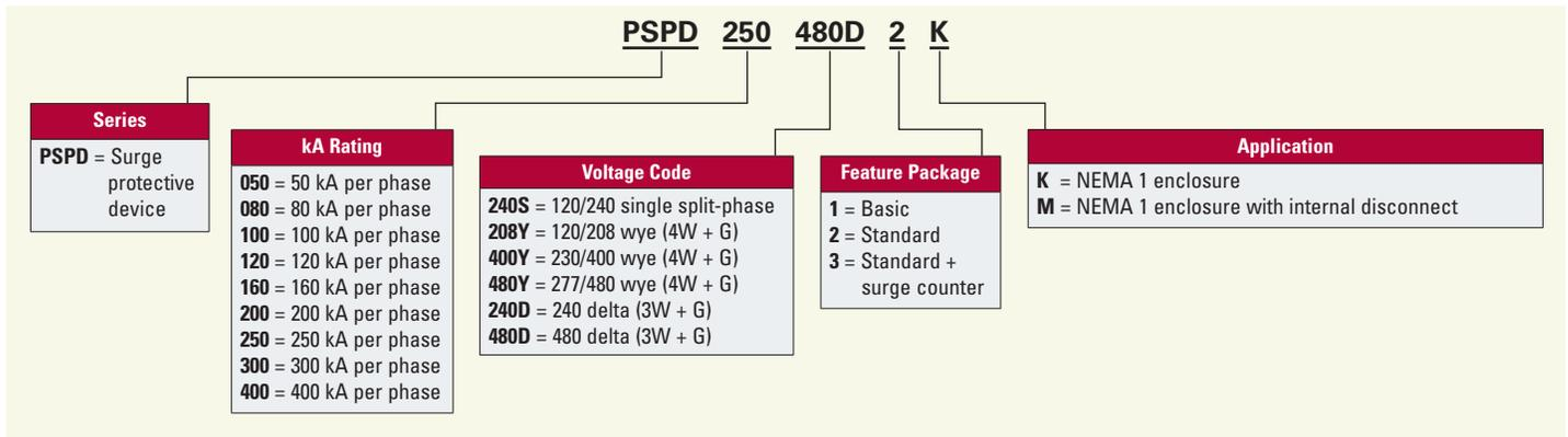
**Example:** PSPD250480D2K = SPD Series, 250 kA per phase, 480D voltage, standard feature package, housed in NEMA 1 enclosure
