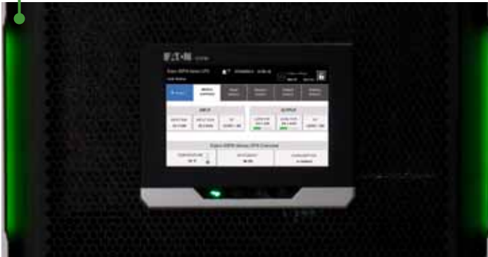
Green light bars showing healthy UPS.
